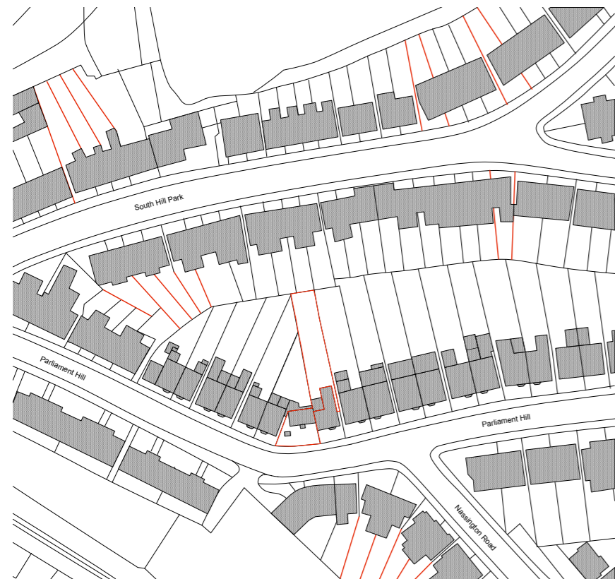
Location Plan: Radial garden walls and plan forms which accord are highlighted in red.
