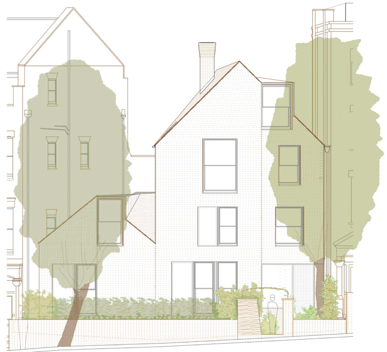
Front Garden Plan & Elevation: Off street parking is removed and the front garden is conforms with the common pattern throughout the conservation area: Brick front garden wall & pedestrian entry gate & path, with front garden planting & light well. The footprint of the house, light well, & line of the entry path follow the root protection zones for the adjacent trees.
