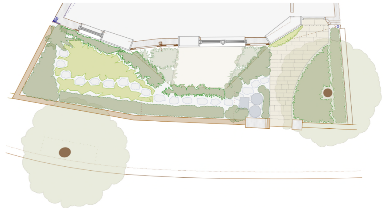
Front Garden Plan & Elevation: Off street parking is removed and the front garden is conforms with the common pattern throughout the conservation area: Brick front garden wall & pedestrian entry gate & path, with front garden planting & light well. The footprint of the house, light well, & line of the entry path follow the root protection zones for the adjacent trees.
