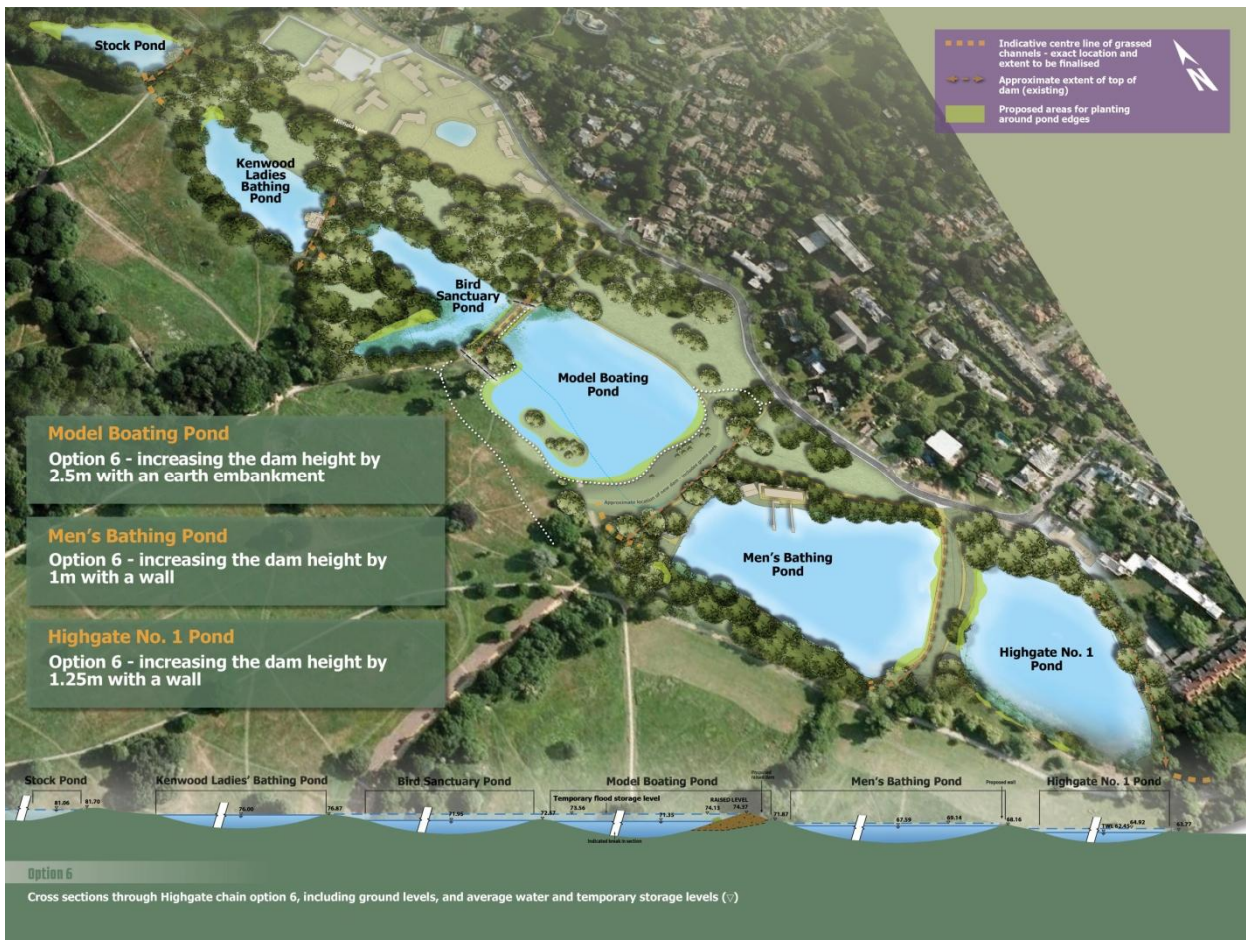
Figure 3.2: Highgate pond chain – proposed Option 6
