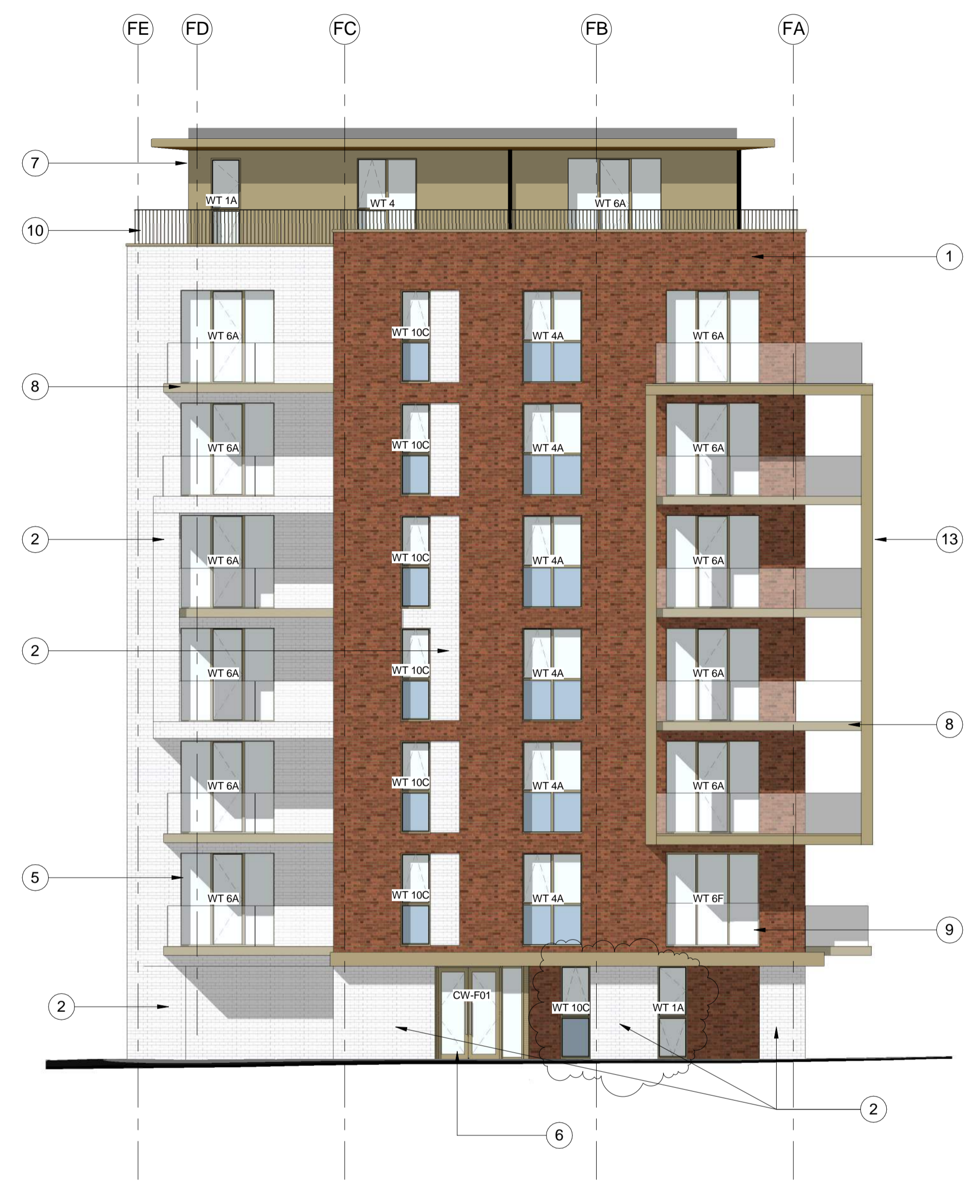
Block F South Elevation 1 : 100
