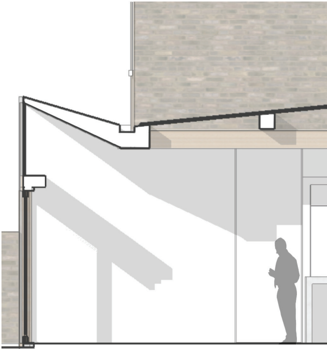
previous rear slope in roof, creating a butterfly shape
