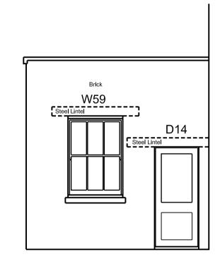
Side Elevation of Rear Extension to No.71 Side Elevation of No.81 Side Elevation of Rear Extension to No.81
