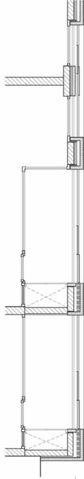
1 Balcony / Sliding Screens Detail
