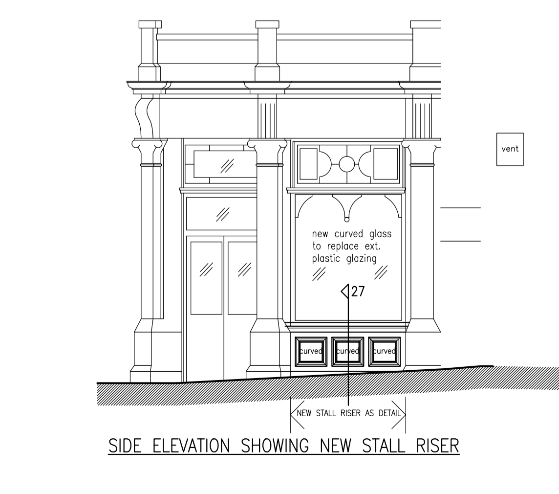
SIDE ELEVATION SHOWING NEW STALL RISER
