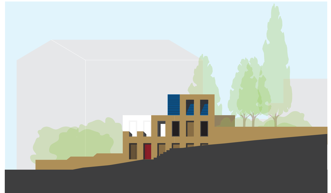
Formative drawing showing the concept of the stepped facade to Streatley Place
