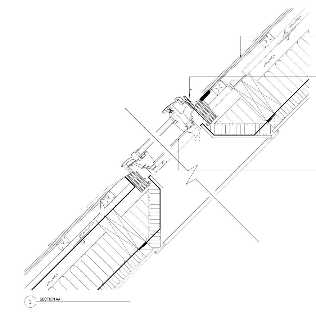
EDN FLASHING KIT - RECESSED INSTALL
