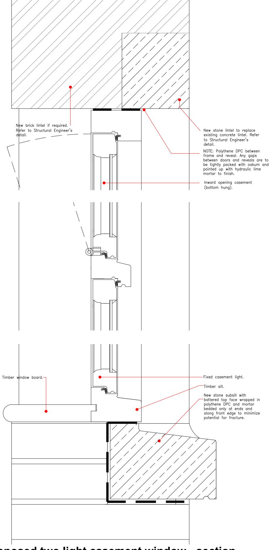
Proposed two light casement window - section Scale 1:2
