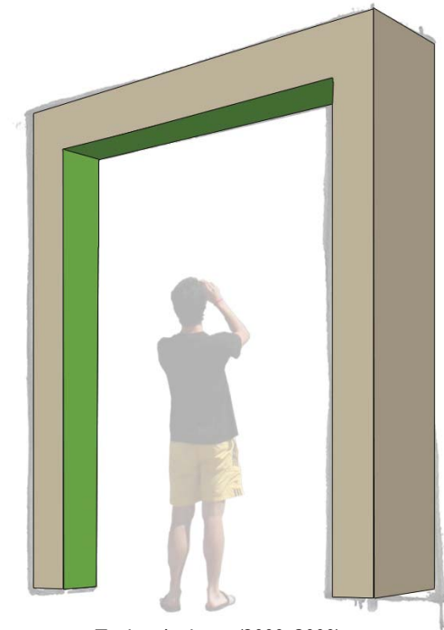
Timber Archway (2000x3000) Material. Scandinavian Pinus sylvestris, metal painted in the inner arch Section size to be confirmed by engineers
