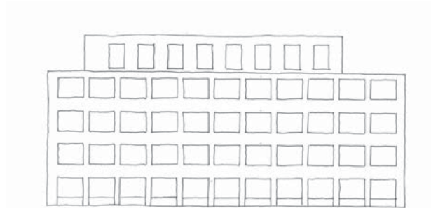
1. Industrial grid - consistent bay widths and heights
