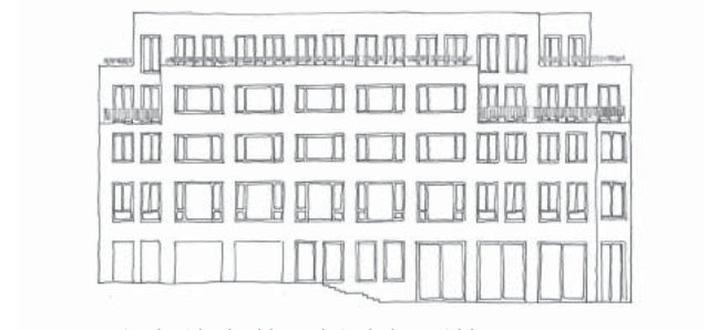
4. Mixed grid - double and single bay widths
