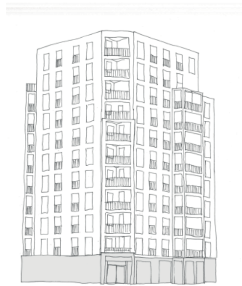
1. Single storey plinth of differing material
