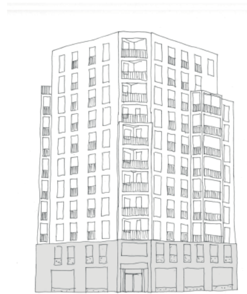
2. Double storey plinth of differing material
