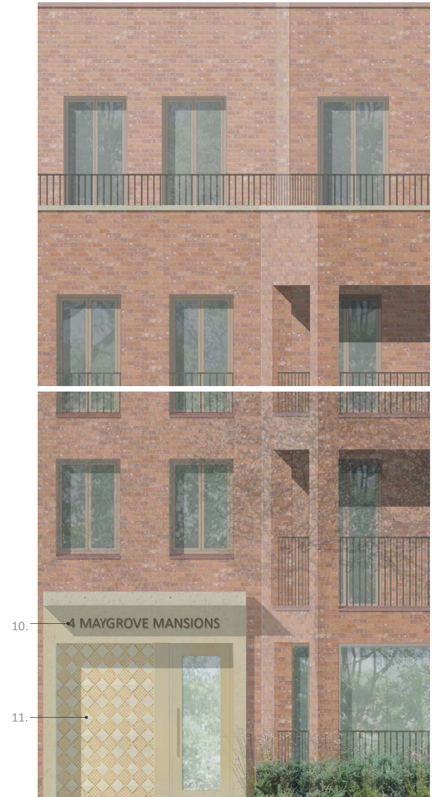
Elevation bay study of south elevation entrance to mansion house
