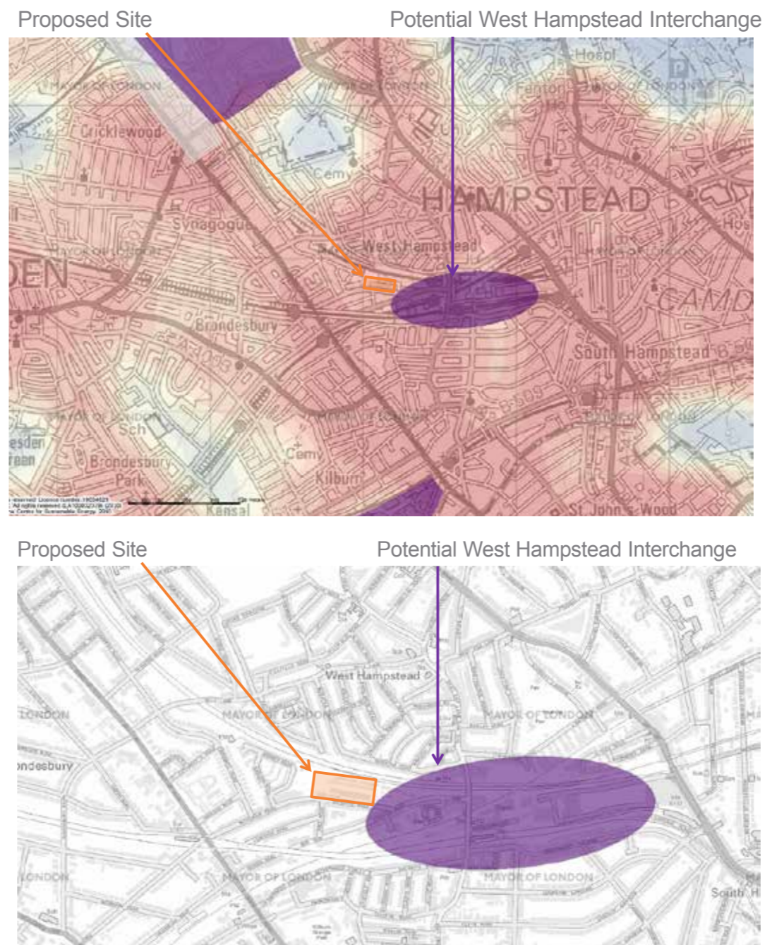
FIGURE 5.4 THE LOCATION OF THE PROPOSED SITE IN RELATION TO THE POTENTIAL WEST HAMPSTEAD DISTRICT HEATING NETWORK (SOURCE: LONDON HEAT MAP)
