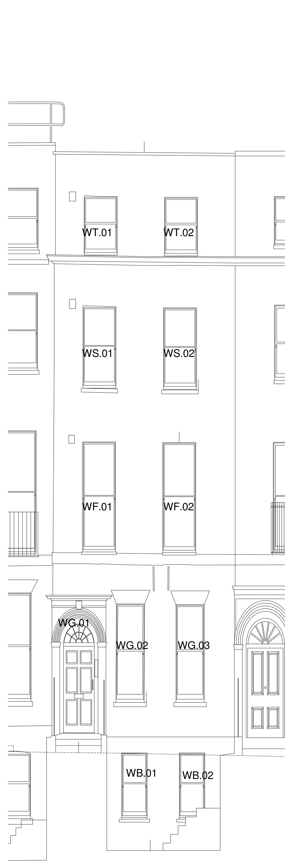
Front Elevation - South - Window Sched. 1:50
