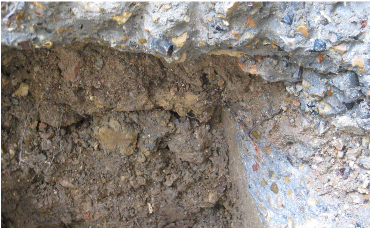
Photograph No. 10 - Trial Hole No. 1 - There were no significant tree roots found within the trial hole, only small fibrous tree roots beneath the concrete sub-base layer of the adjacent conifer tree.
