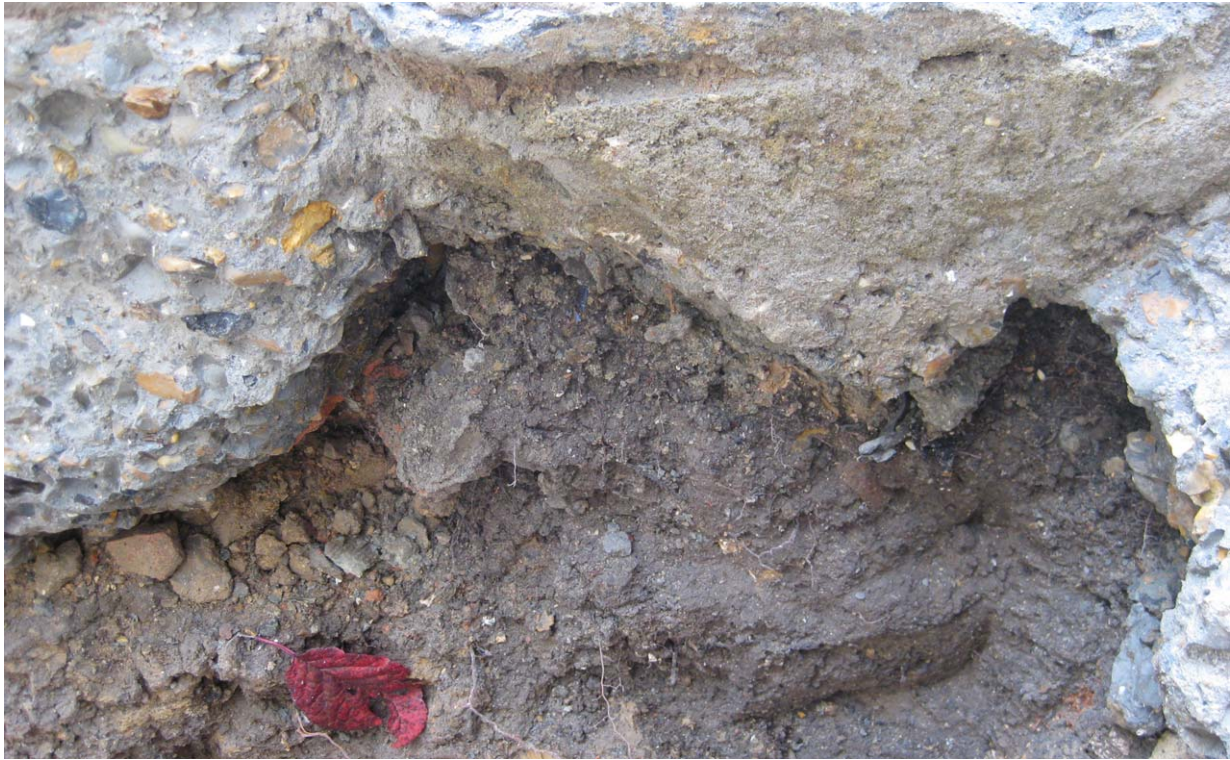
Photograph No. 13 - Trial Pit No. 2 - There were no significant tree roots found within the trial hole, only small fibrous tree roots beneath the concrete sub-base layer of the adjacent plum tree.
