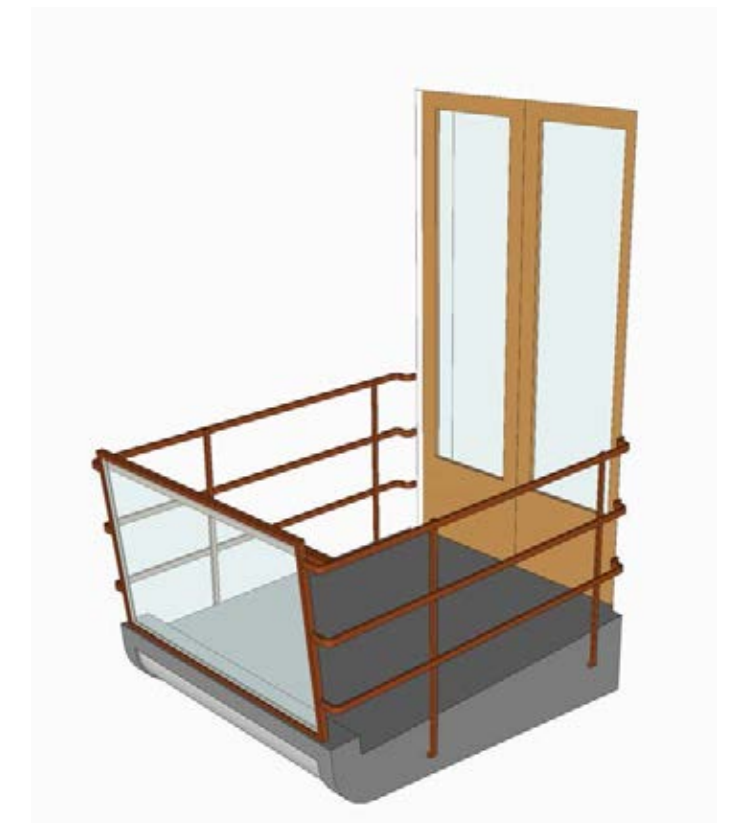
Proposed balcony with penny bronze balustrades and framed glass front panel. Redundant lighting is removed
