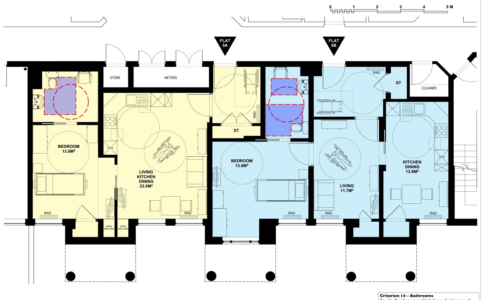
Principle: Provide an accessible bathroom that has ease of access to its facilities from the outset and potential for simple adaptation to provide for different needs in the future.
