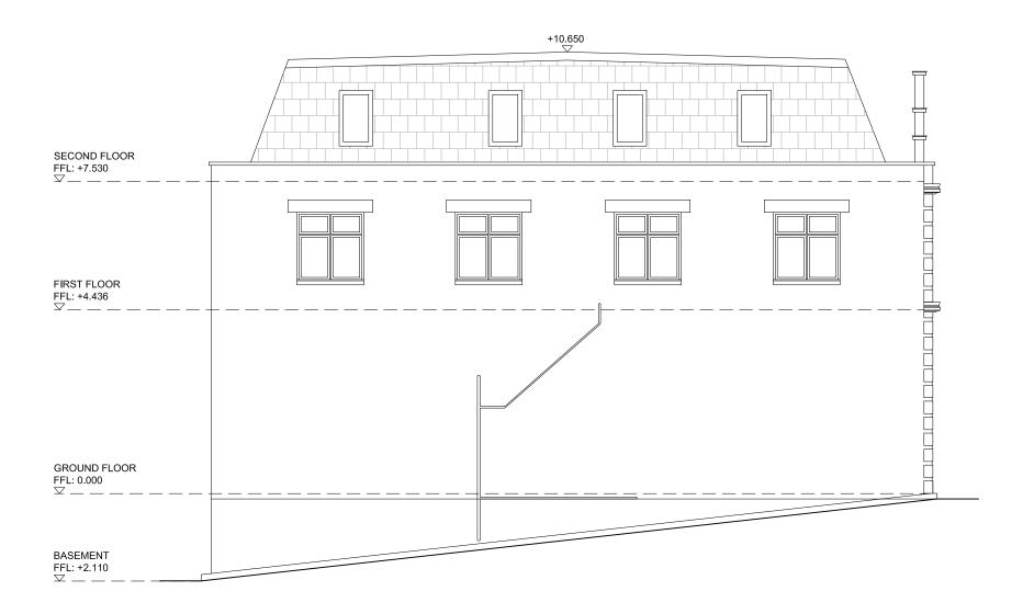
**Existing South Elevation** SCALE 1:50 @ A1 / 1:100 @ A3
