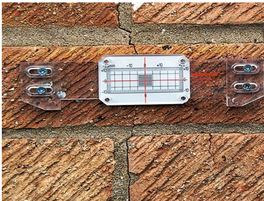
Figure 1: Typical Avonguard Tell-Tales monitoring gauge
