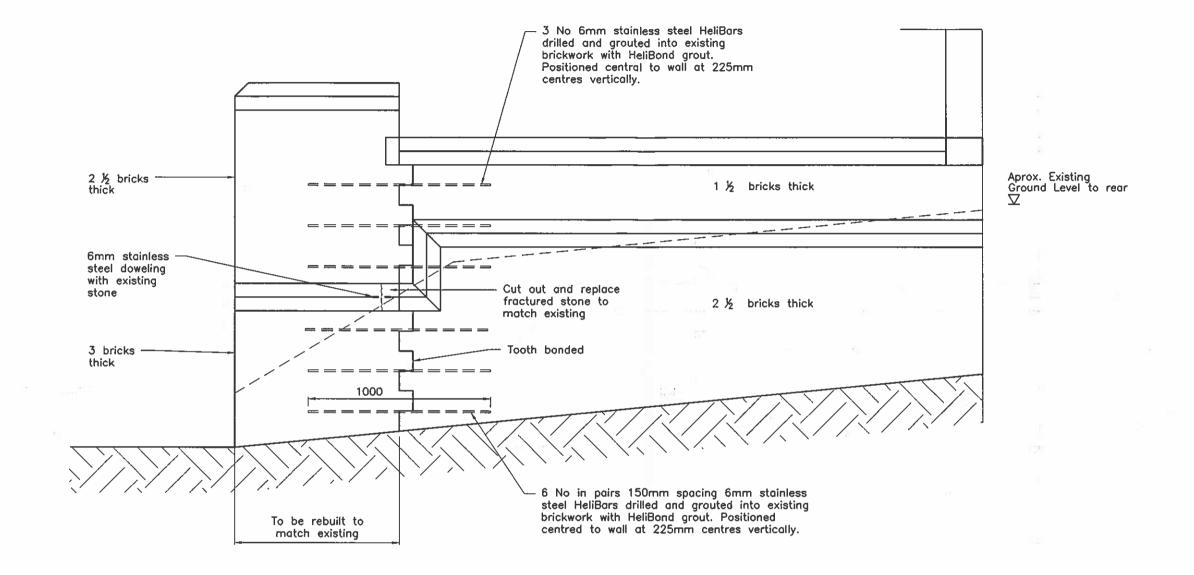
Carefully demolished existing brick pier cleaning and keeping existing bricks for reuse. Replace broken bricks with new secondhand to match. Rebuild with traditional line mortar to match existing.
