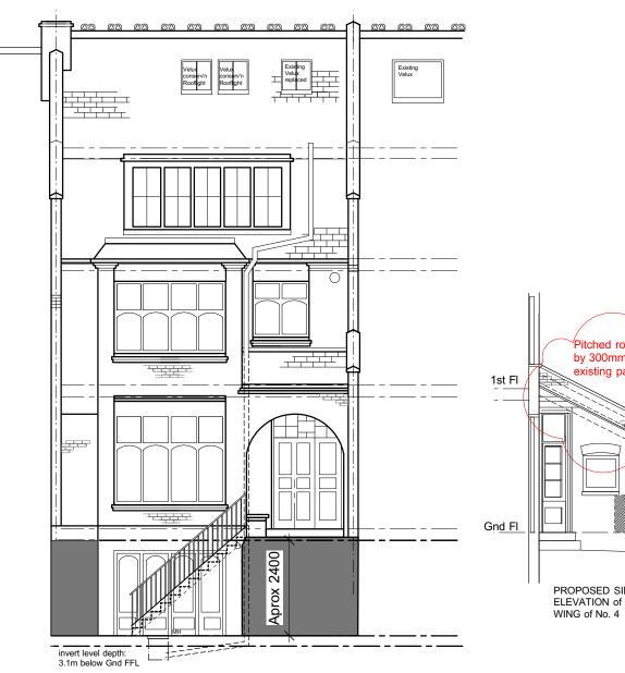
Pitched roof of No 6 rasied by 300mm but still below existing party wall parapet PROPOSED SIDE ELEVATION of CLOSET WING of No. 4
