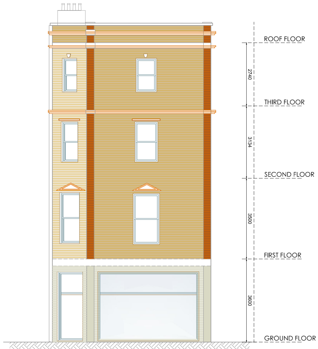
EXISTING FRONT ELEVATION
