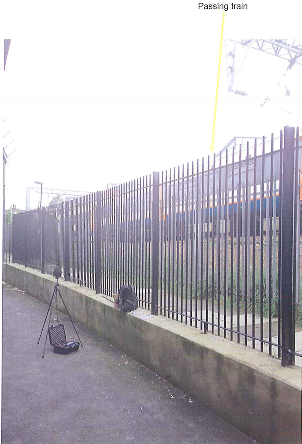
PHOTO C: Microphone located next to railings with railway line behind
