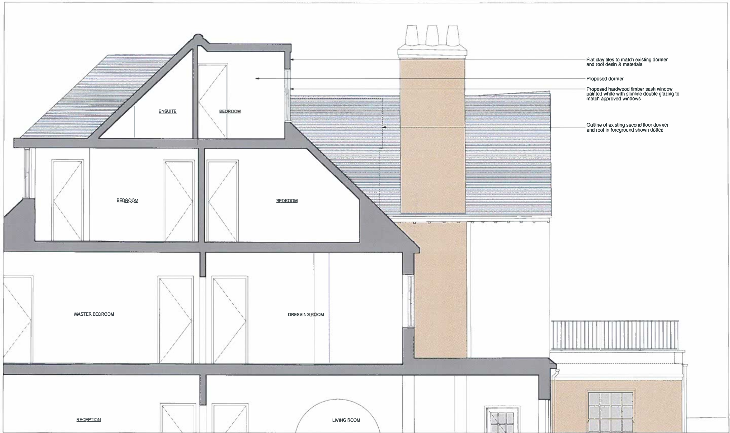
01 Proposed Dormer - Section A GS.01 1:50
