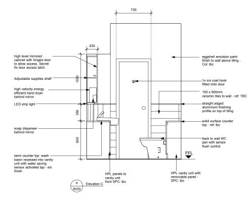
Note: Typical elevation layouts and finished from R.B.13 to match R.B.11
