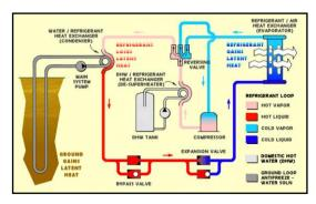
a heat pump, an air delivery system (ductwork), and a heat exchanger-a system of pipes buried in the shallow ground near the building. In the winter, the heat pump removes heat from the heat exchanger
