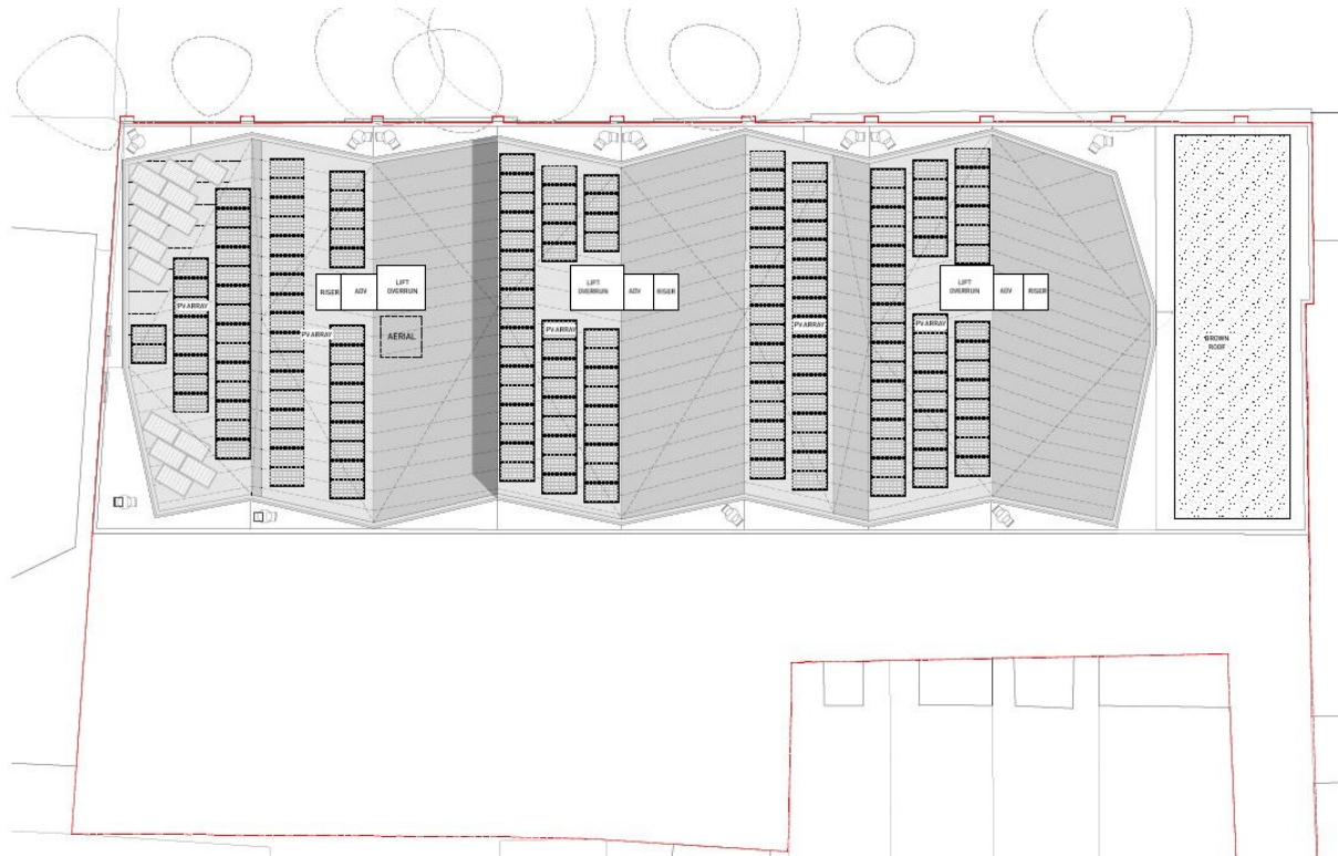
Figure Proposed PV panel installation by Architects
