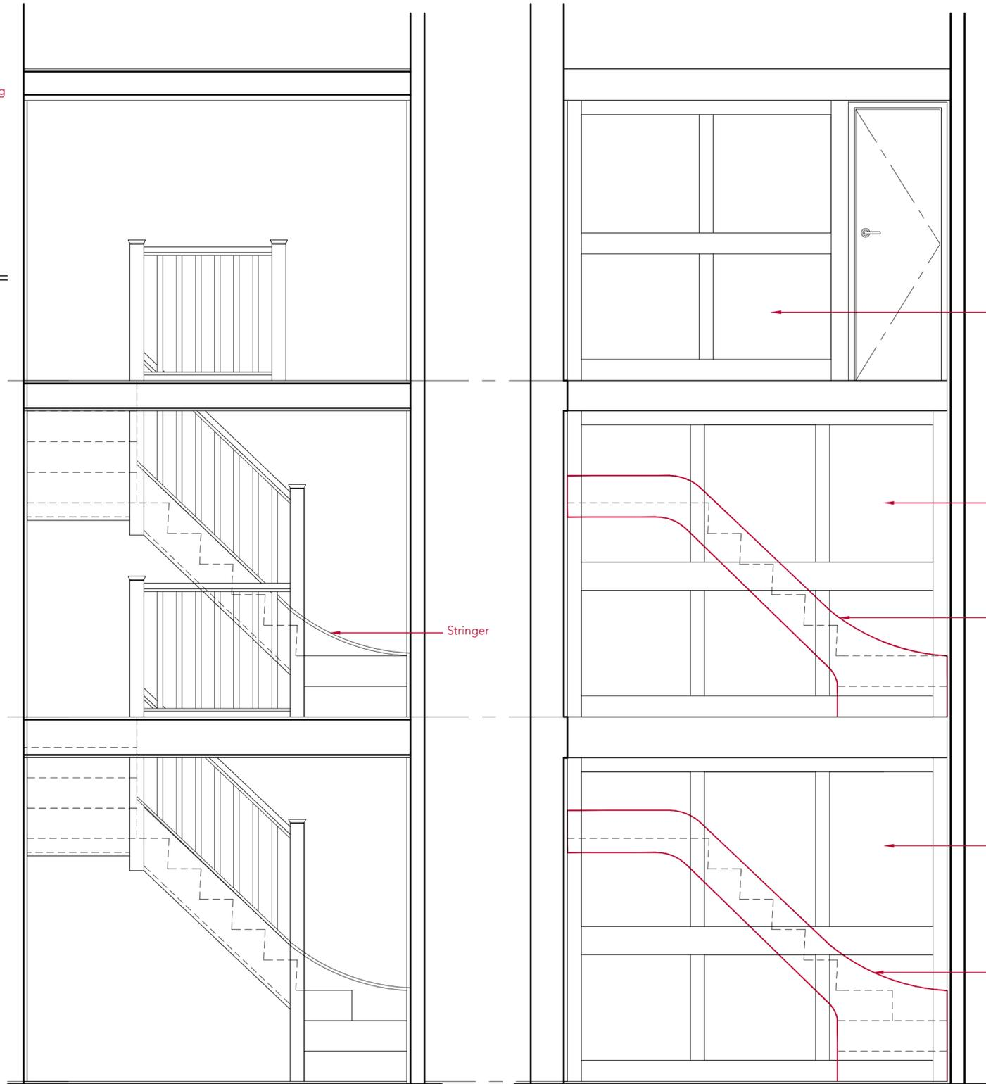
4 Elevation for Staircase scale 1:25
