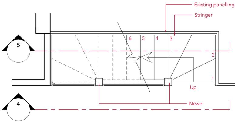
1 Details plan for Ground Floor Staircase scale 1:25
