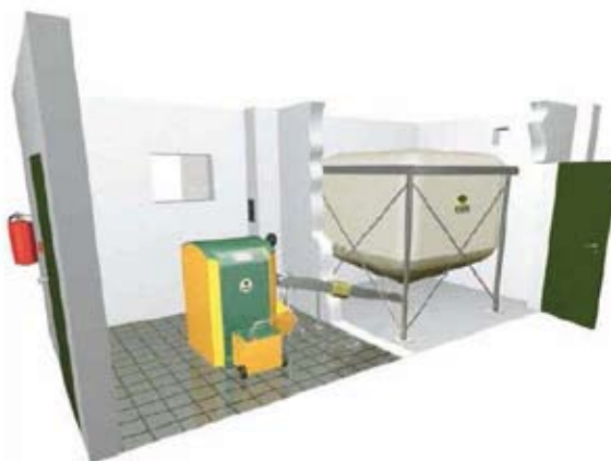
Example of pellet boiler and pellet storage room. Source: Energy Crops Limited
