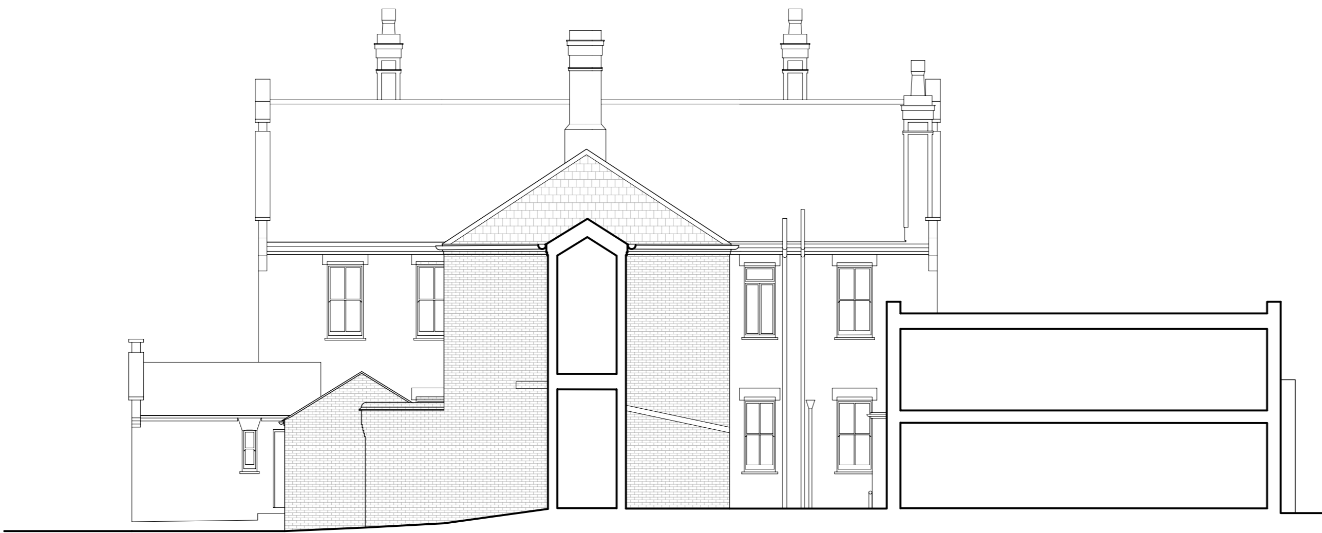
EXISTING ELEVATION 09 (South facing section / elevation through existing south building with Holmes Road front building beyond)
