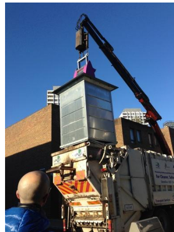
Photo 4: Special waste vehicle in process of emptying a SULO underground waste container.
