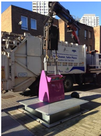
Photo 3: Special waste collection vehicle in process of lifting a SULO underground waste container out of the ground.
