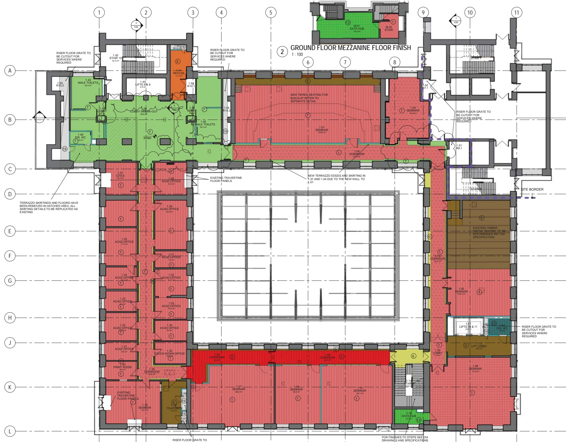
1 PROPOSED LEVEL 1 FLOOR FINISHES PLAN 1:100
