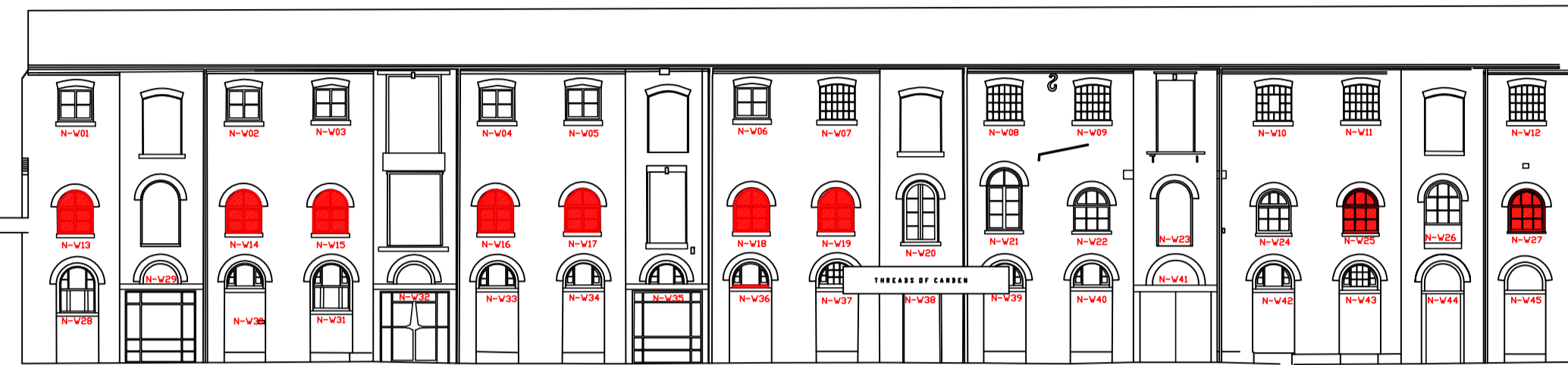
NORTH ELEVATION Windows of this type highlighted in red are proposed to be replaced.
