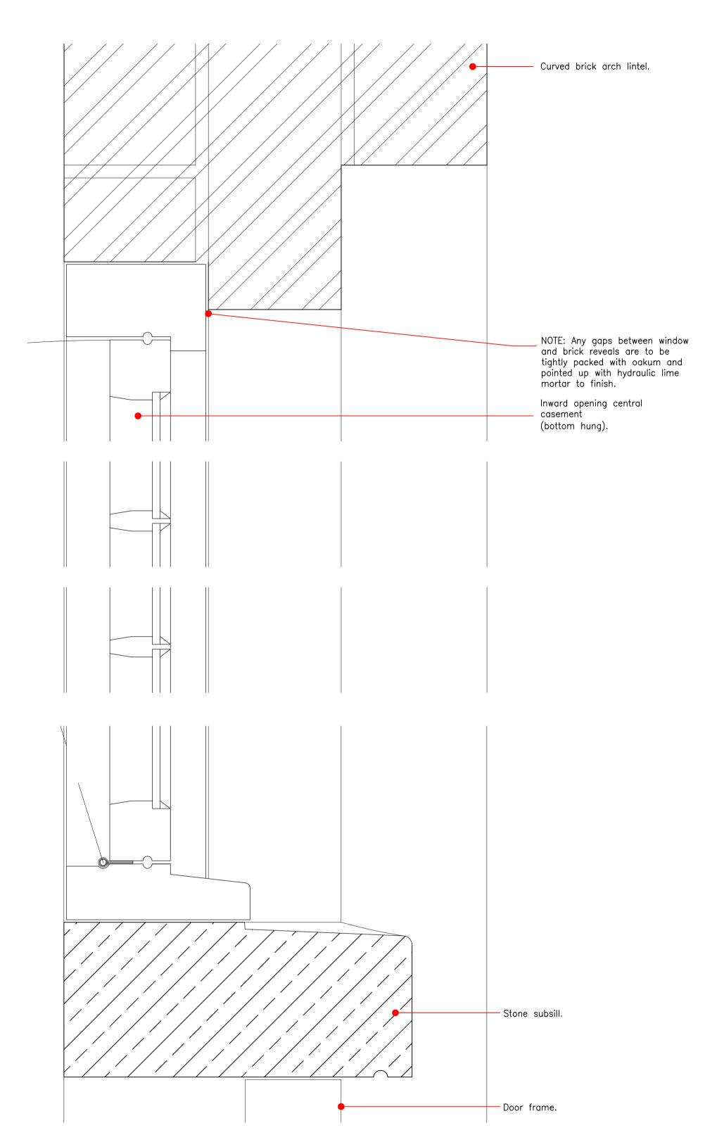
Existing fixed light / opening casement timber window - section Scale 1:2
