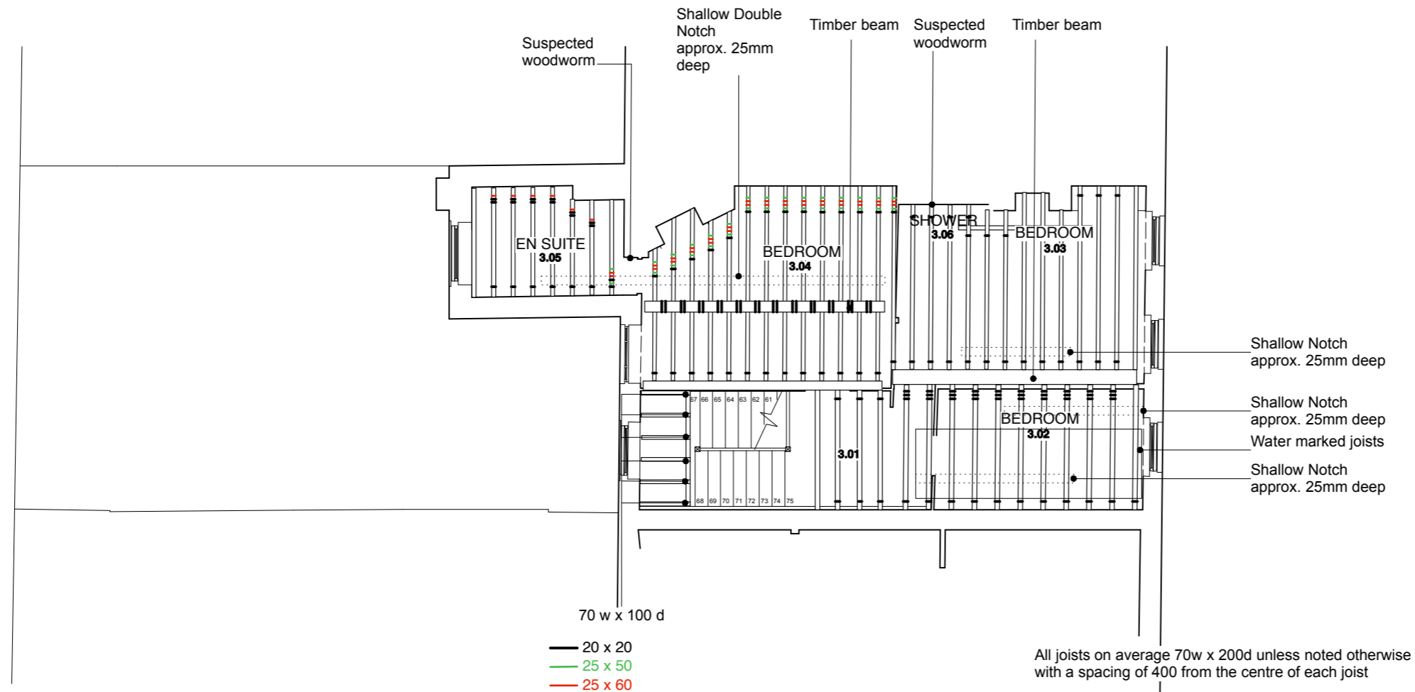
PROPOSED THIRD FLOOR PLAN SHOWING FLOOR JOISTS
