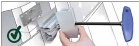
Only with a limitation to 12 - 14 Nm!
