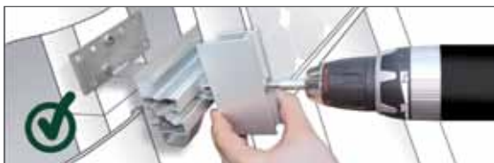
Only with a limitation to 12 - 14 Nm!
