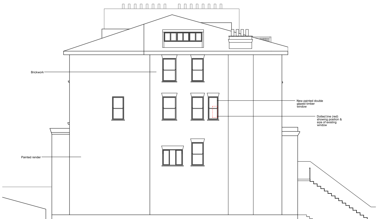
Proposed side elevation showing the new window opening at No. 17 Belsize Park Gardens
