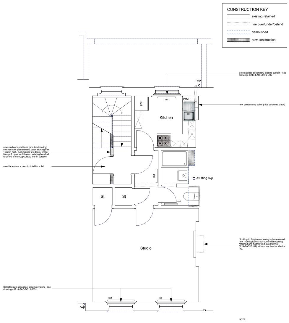
All ceiling plasterboard to be replaced throughout the second floor (1 hour fire resisting) on resilient bars.
