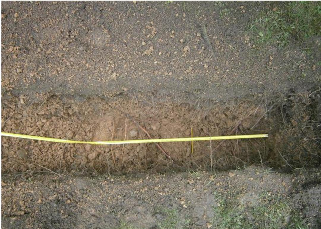
Photograph 14. Trench 2: Roots between 150mm and 600mm depth.
