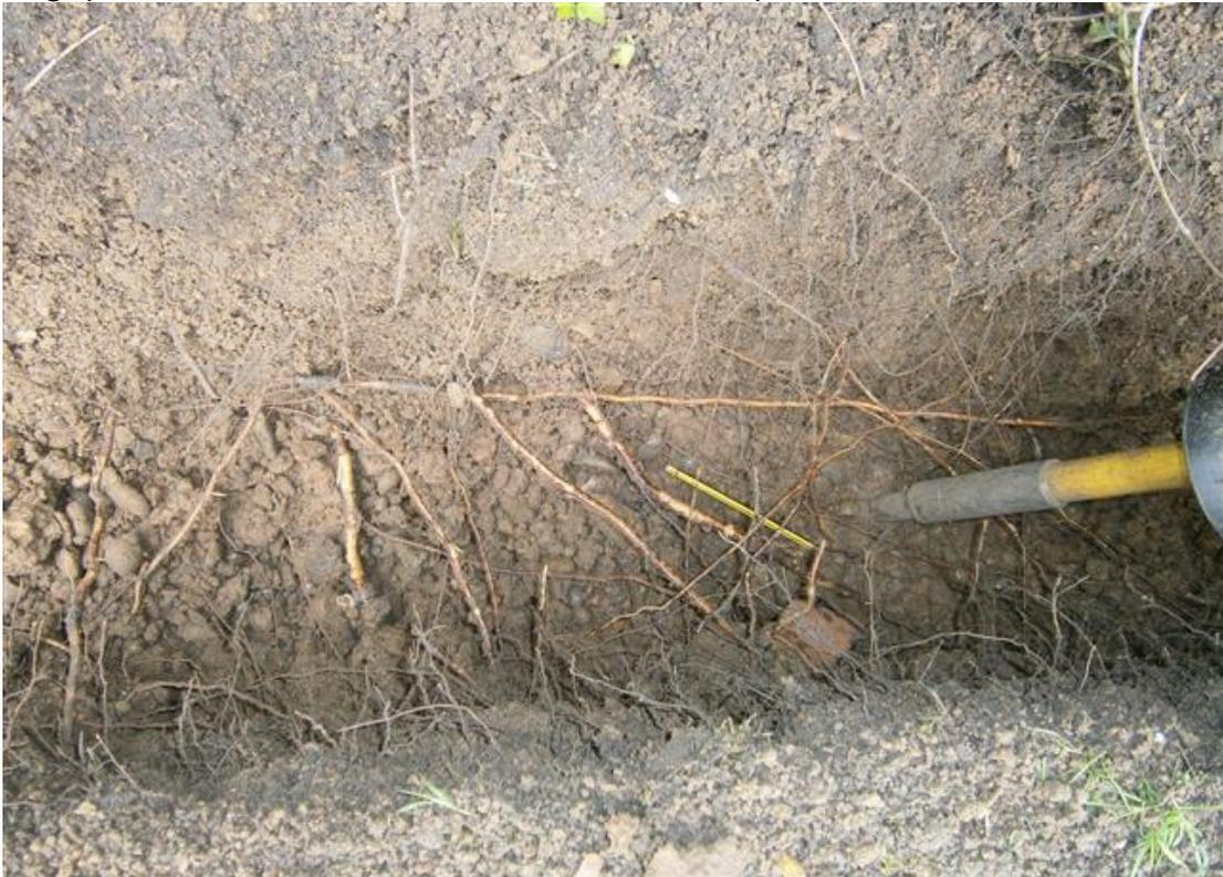
Photograph 6. Trench 1: Roots between 150mm and 600mm depth.
