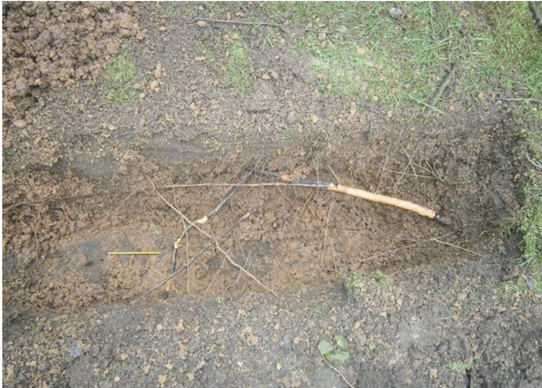
Photograph 21. Trench 3: Roots between 0mm and 600mm depth.
