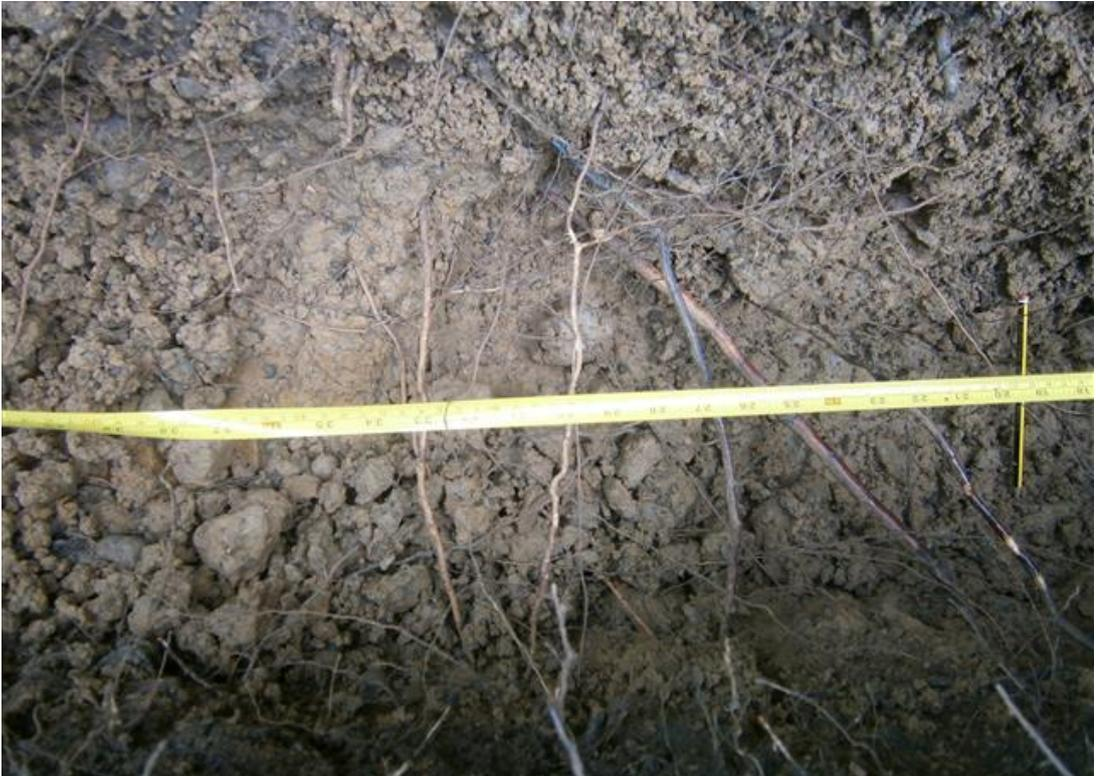
Photograph 16. Trench 2: Roots between 150mm and 600mm depth.
