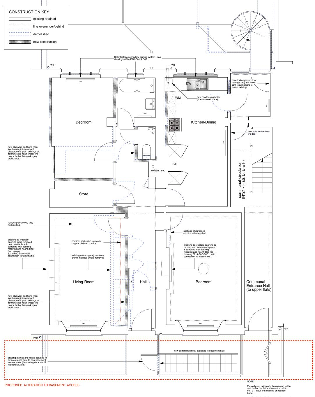
All internal doors to be replaced with solid timber flush fire doors except bathroom door (fully glazed with white/obscure laminated glass - for borrowed light into hall).
