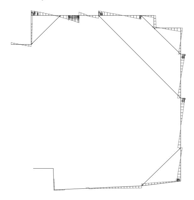
Maximum Shear force in this diagram is 1800kN
