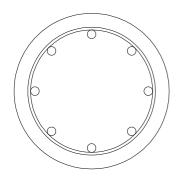
600dia. RC Pile 8T25 Vertical T8@150 Transverse
