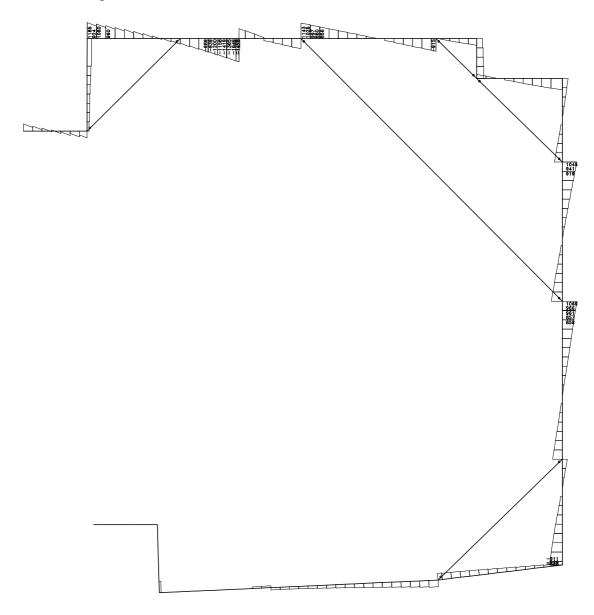
Maximum Shear force in this diagram is 1700kN
