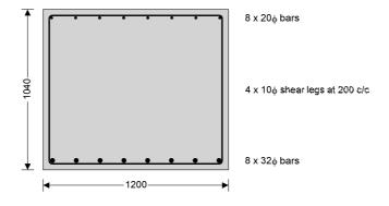
Rectangular section in flexure (Section 6.1) - - Positive midspan moment
