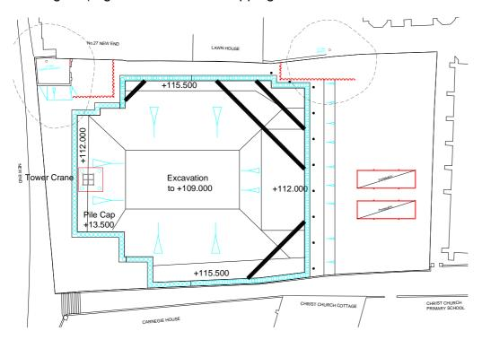
• Stage 5 (Excavation of North and south berms to +109m and East West to 112m level, casting the center slab, new rakers at +116m and +112.5m)
