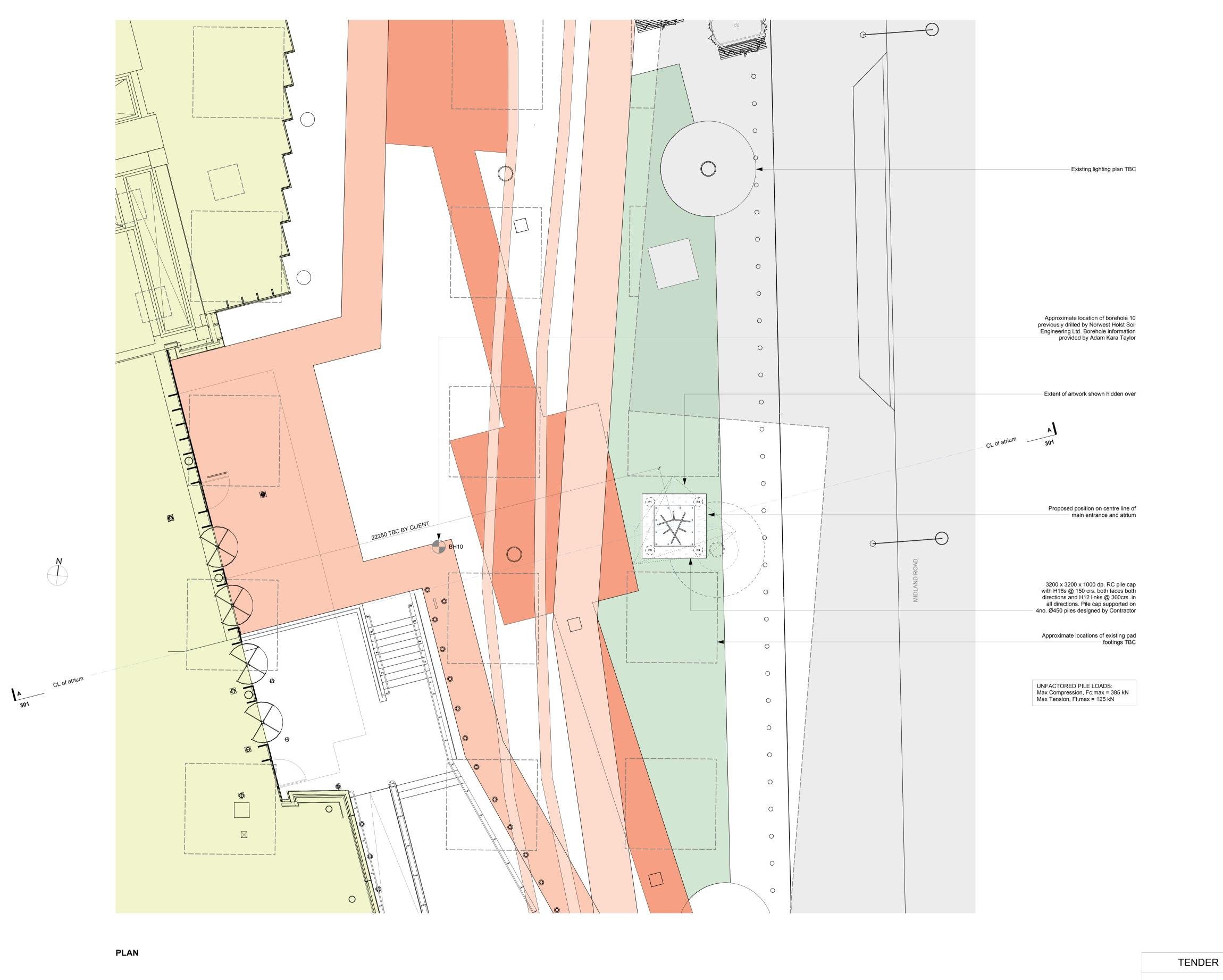
Reinforced concrete foundations Preferred artwork position Constraint: ThamesLink box under
