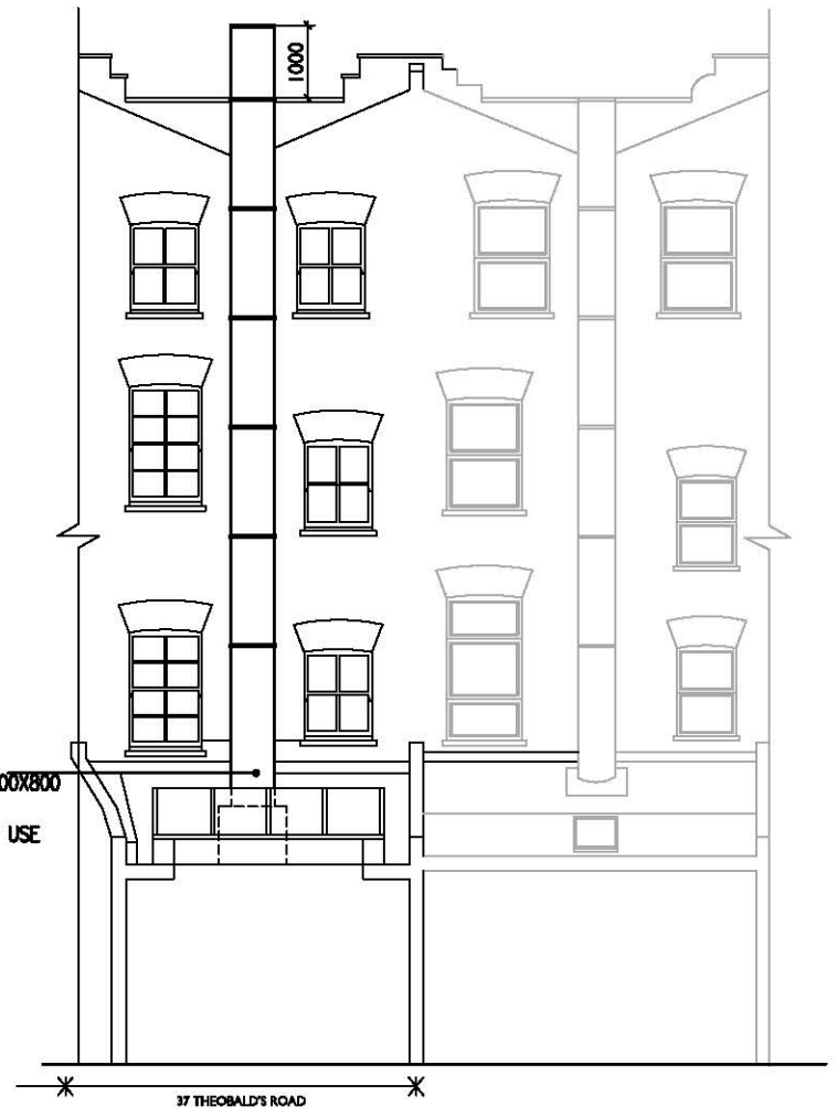
PROPOSED REAR ELEVATION
