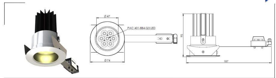
A new low cost, high specification fixed LED downlight offering the very best LED package in a classic Light Corporation designed downlight. The light source is set behind a black anti-glare baffle to reduce peripheral sparkle. Available with 12°, 19° or 36° optics. The SRF can be specified to take a sandblasted diffusion lens increasing the IP rated to IP54, softening lens, coloured filter or honeycombe louvre if required.
