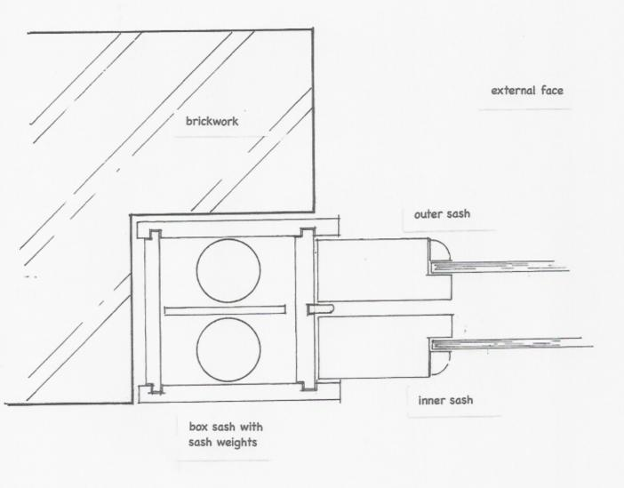
section showing recessed box sash to existing sash windows in front elevation
