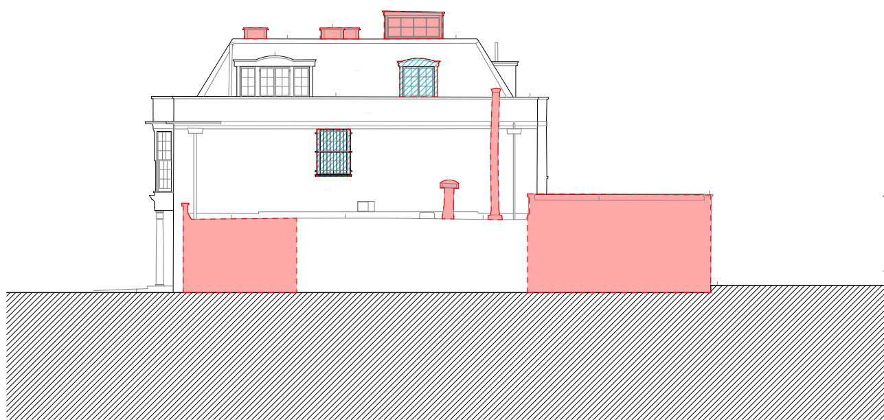
SIDE (EAST) DEMOLITION ELEVATION
