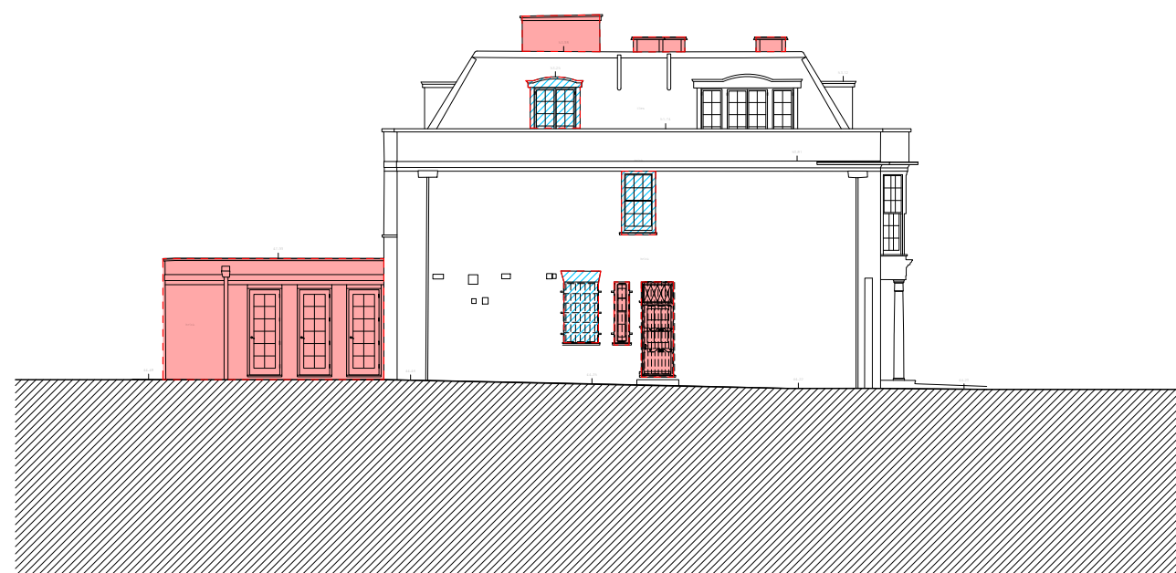
SIDE (WEST) DEMOLITION ELEVATION
