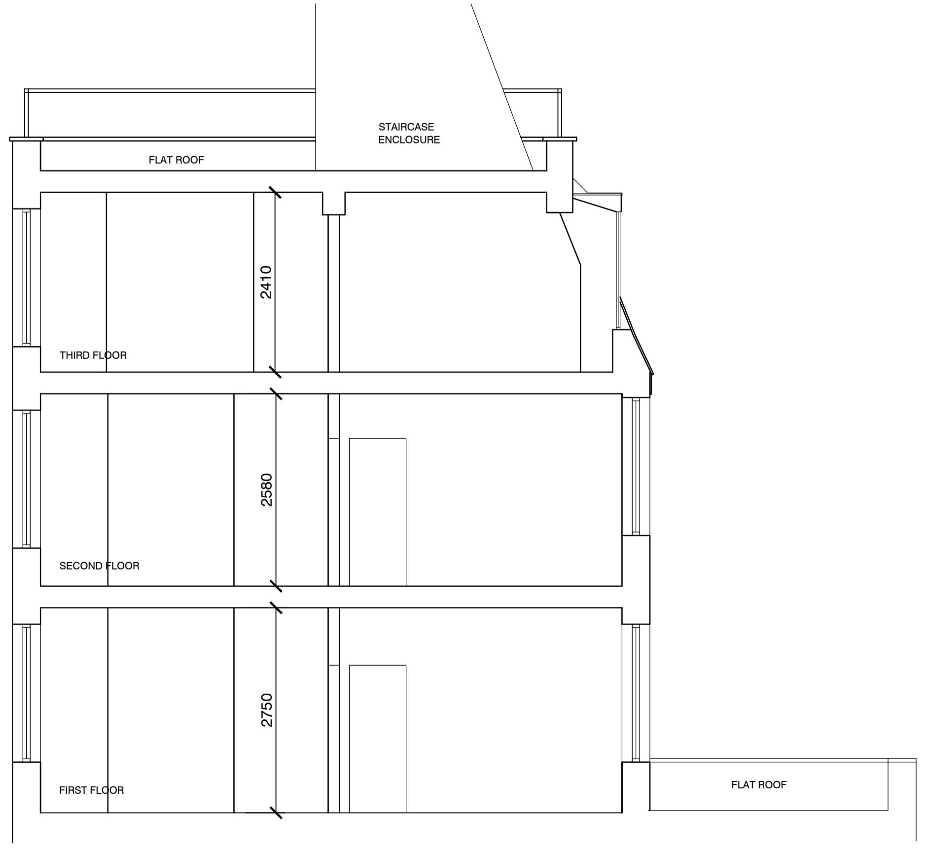
SECTION THROUGH-UPPER FLOORS
